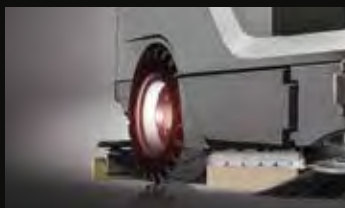
Rear/front super elastic wheels kit, for minimal vibration and increased comfort
